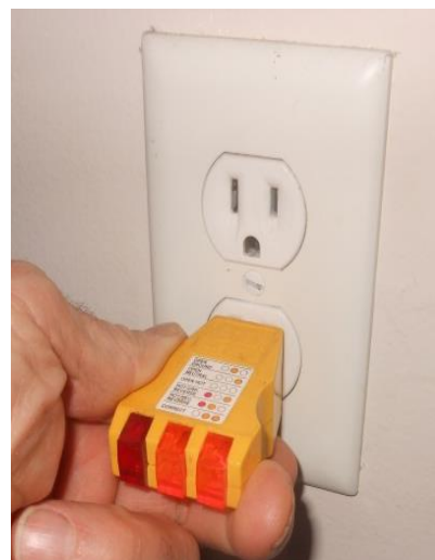
Checking walls: Measure the cavity and the existing insulation level. Make sure wall outlets work before and after insulation installation.
