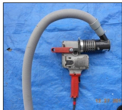
Lead-safe drilling: Using a shrouded drill with a HEPA vacuum removes dust where it is generated.
